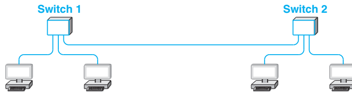
Figure 25.4 Four hosts connected by two switches.
