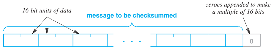
Figure 8.9 The Internet checksum divides data into 16-bit units, appending zeroes if the data is not an exact multiple of 16 bits.
